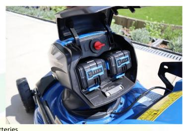
With many manufacturers the batteries can be shared across a range of power tools including grass trimmers, hedge trimmers, leaf blowers etc. This means that you have the option of purchasing the cordless lawn mower with no batteries (bare tool), if you already have a battery and charger available. This will save significantly on the cost when purchasing.
