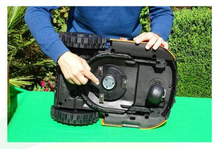
cleaning as lots of grass clippings and debris will get lodged in the wheels and around the blade. Not only does this affect the speed and performance of the robot mower but it will also force your mower to use more power. This will increase how often your mower needs to charge and will reduce the quality of the cut. It's just not worth it.
