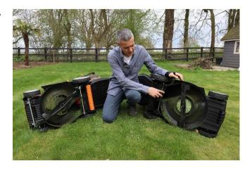
Rotary blades need to be sharp in order to provide a clean and precise cut of the grass. They can be easily sharpened and when required, are low cost and easy to replace.
