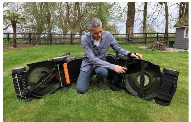
Rotary blades need to be sharp in order to provide a clean and precise cut of the grass. They can be easily sharpened and when required, are low cost and easy to replace.
