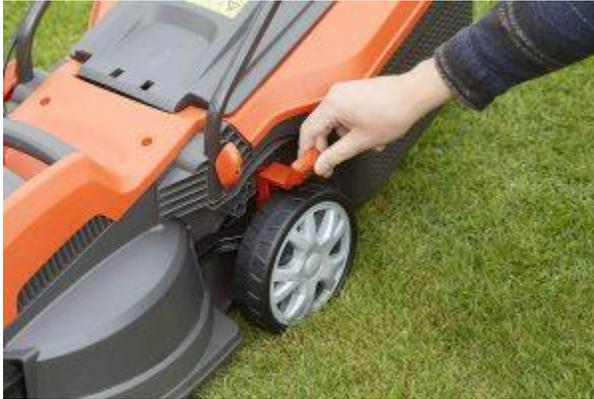
In order to combat the changing season and to continually improve the look of your lawn, you can adjust the height at which the Flymo Speedi-Mo 360C cuts at. This is done very easily using the large lever located on rear/side of the mower.
