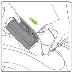
Ensure the 'G' logo is facing upwards when you slide the battery into the battery housing. It will click into place once fitted correctly.
