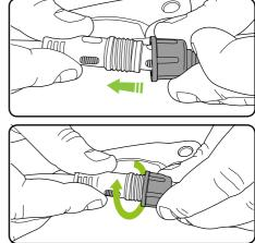
Slide the collar over the power cables. Screw the collar in a clockwise direction to tighten. Thread until tight.
