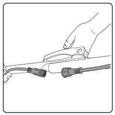
The power cables are located below the locking handle on the left side of the mower's handle.
