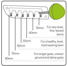
The mower has 6 cutting height settings between 30mm and 80mm.
