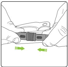
Push the power cables together until they lock in place.
