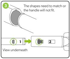
When the pole is fully inserted, the button (1) will pop up into the aperture (2)
