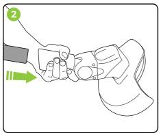
Insert the body pole into the grass trimmer head, ensuring it is the right way up.
