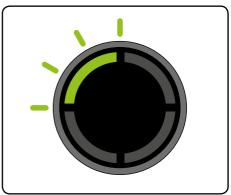
When there is no power left the final LED will flash for 10 seconds and then go out.
