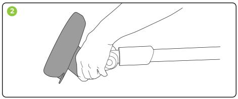
The head only rotates in one direction.
