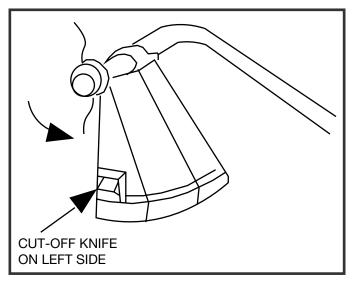
For nearly all cutting, it is good to tilt the line head so that contact is made on the part of the circle where the line is moving away from you and the debris shield. The results in the debris being thrown away from you.
