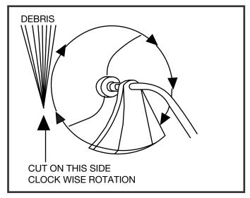
Line head rotates in a clockwise direction when looking from above. The cut off knife will be on the right side of the debris shield.
