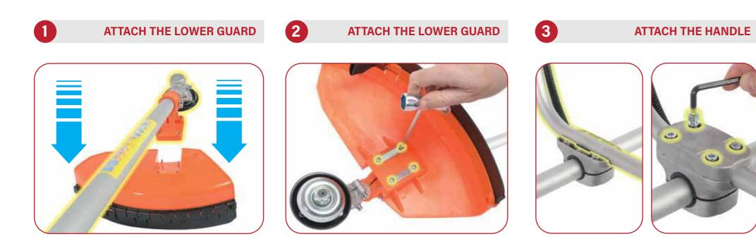
Attach the guard to the lower shaft using the screws and tools provided.
