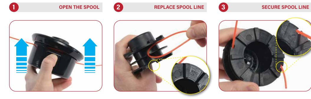
Open the spool by pressing one of the two clips to loosen the cover. Once loose firmly press the second clip and remove the spool cartridge from inside the housing. Secure the replacement spool line to the cartridge as shown The cartridge consists of two compartments in which the spool line needs to be wound. Wind in the direction shown on the body of the cartridge. Secure the spool line inside one of the two lugs on the body of the cartridge to prevent it unwinding.
