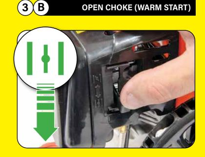
For warm engine starts open the choke by sliding the lever downwards.
