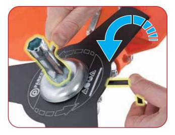
Place the allen key through the locating hole of the collar, through the hole of washer "A" and into the hub.
