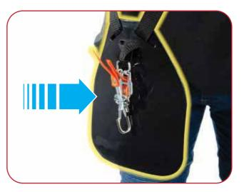
Ensure the thigh pad is located in the correct position so it protects you fully from pressure points created from contact with the machine during use.
