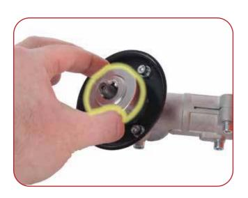
Install washer "A" as illustrated above. Align the hole in the washer with the hole in the spool collar. This is to help you lock the hub with an allen key later on in the process.
