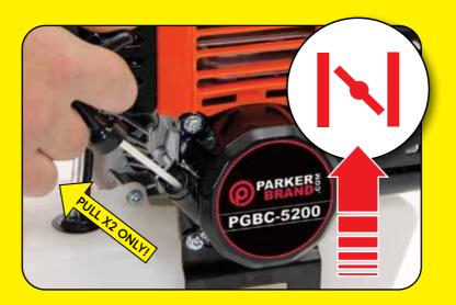
Make sure that the choke is <u>CLOSED</u> (UP **CLOSED POSITION**)
