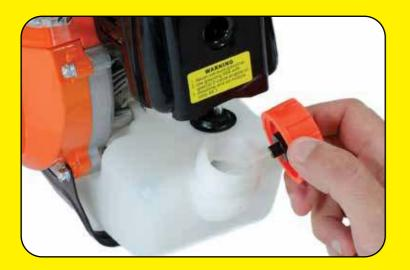
Remove the fuel cap and fill the tank to no more than 80% capacity.
