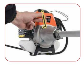
Tighten all the bolts with the allen key provided in the tool kit.
