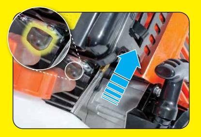
Prime the carburettor by pressing the primer bubble located underneath the air filter housing.
