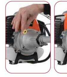
Finger tighten a bolt in one of the top bolt holes, then one in the diagonal opposing bottom hole.
