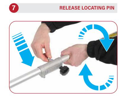
Twist to release the pin and rotate the lower shaft until the pin locates into the location hole.
