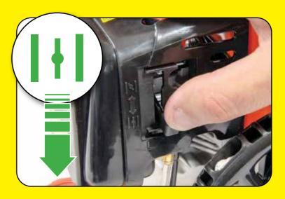
Make sure that the choke is <u>OPEN</u> (DOWN **V** OPEN POSITION)
