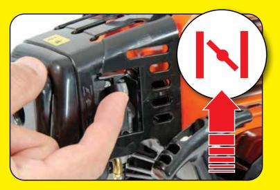
For cold engine starts close the choke by sliding the lever upwards.
