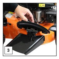
6.31 Lower the side discharge flap so it rests on the top of the side discharge chute (1).
