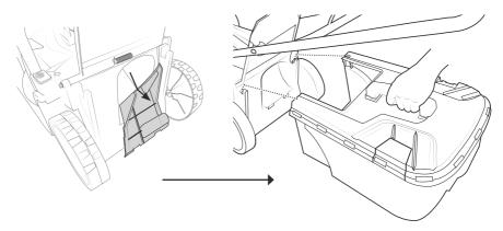
**NOTE!** If you wish to collect the grass in the Collection Basket, ensure the Mulching Accessory is removed first.
